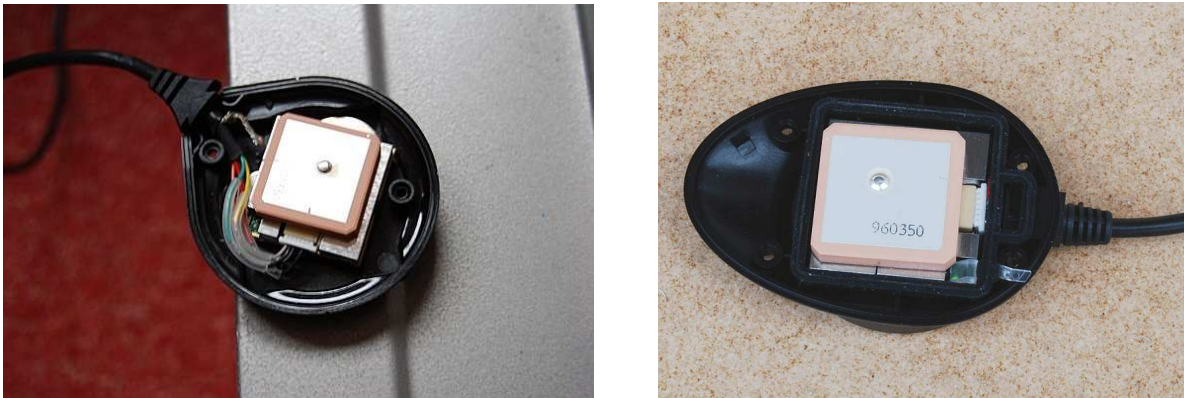
Figure 34: An EM-406A module embedded into the housing of a Fortuna U2, to the left, and embedded into a housing of a Navilock NL-303P, to the right.
