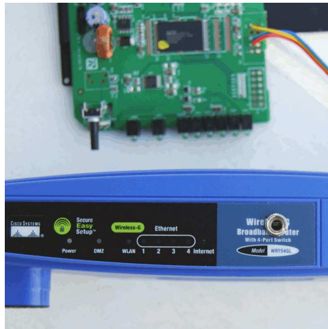
Figure 40: A modified Linksys WRT55GL router.
